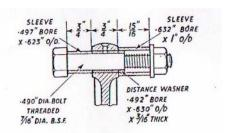
RE-ADJUSTING THE PEKING BOLT Fig 2.
