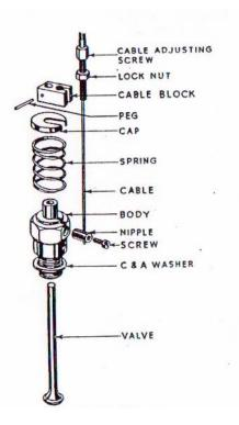
EXPLODED VIEW OF THE DECOMPRESSOR Fig 3.
